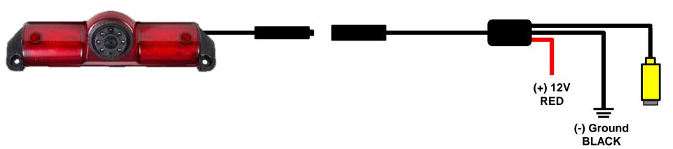
RED WIRE: Connect to 12V+ power source (ACC or IGN or REVERSE)
