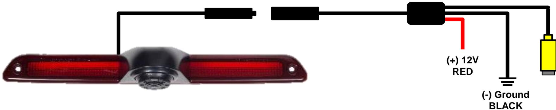
RED WIRE: Connect to 12V+ power source (ACC or IGN or REVERSE)
