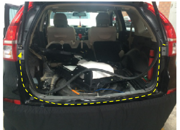
Rear Seat Release Handle Mounting Location
