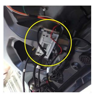
Locate the OEM outside opener switch connector, on the rear of the switch assembly. Disconnect the OEM connector, and connect our T-Harness in line with the outside opener switch.
