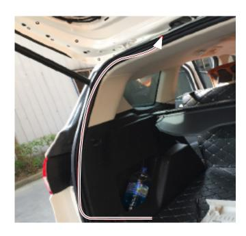
17. Using a wire puller or fish tape, pull the wiring harness through the factory wiring boot into the liftgate structure.
