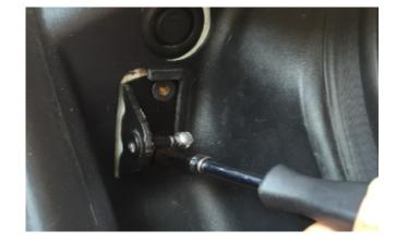
10. Install the supplied Power Lift Gate Motors, noting the Left and Right orientation as marked on the motor assemblies. Mount the motor with the wiring harness towards the upper (lift gate) side.
