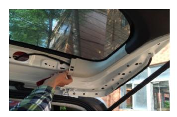
3. Using a moulding remover, carefully pry on the handle cover to remove it and expose the screws. Remove the 2 screws underneath the cover.
