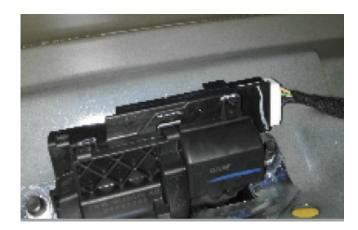
15. Locate the control module in the mounting location. Note that the supplied bracket will line up with preexisting holes in the lift gate body structure. Mount the control module as shown.
