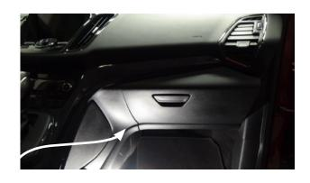
25. Connect the Power Lift Gate's power wire to the red wire at the rear of the fuse panel with the supplied connector clamp.
