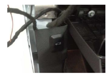
**NOTE**: Higher trim level vehicles will use the OEM button, located to the left of the headlight control switch (pictured). If the OEM switch is present, the supplied button is not used and no connection to the kit is requred. Trunk signal is detected through the CANBUS connection.
