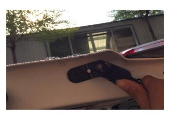
Remove the 2 screws and then remove the LH side mounting ball and bracket for the OEM gas support strut. Replace with the one included in the kit.
