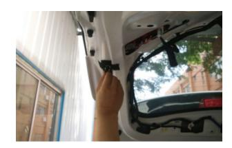
13. Visually inspect and identify the LEFT and RIGHT side lift motors, as marked on the new power lift motors. Install the new lift motors to the correct LEFT and RIGHT sides, with the wire harness of the lift motor directed towards the body of the vehicle.
