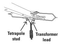
Use them to attach the transformer to the bottom of the antenna at the studs on tetrapole.
