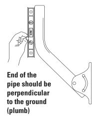
Secure the foot to its permanent location. Adjust the end of the pipe so that it is perpendicular to the ground. Tighten the hex nuts to hold the pipe in place.
