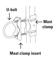
Find the U-bolt and mast clamp insert (see the illustration to the left). Put the U-bolt into the mast clamp insert with the teeth of the mast clamp insert facing the closed end of the U-bolt.
