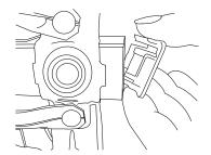
Insert the plastic end caps in the ends of the booms as shown here. Use a rubber mallet to gently tap them into the antenna booms to secure them.
