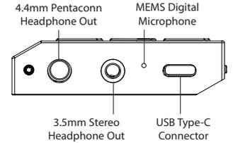
Fig. 1 Connector Panel on M200
