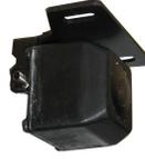
10. Find a suitable location on the vehicle where the bracket will not interfere with any equipment or doors, or block the line of sight. Verify that the planned mounting location is accessible from behind and that you have access to route the wiring inside the vehicle. Be sure that the mounting screws will not hit any wires or equipment inside the vehicle.
