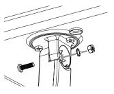
4. Attach the arm to the base. Find one of the screws, washers, and nuts included in the package.
