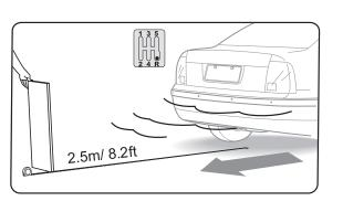
After installation is complete you should test the system. With the vehicle on a flat surface with no obstructions (not inside the shop), ignition OFF and parking brake engaged. Turn the ignition on and have someone inside the vehicle place their foot on the brake and shift the vehicle to Reverse. Stand to the side of the vehicle and place your hand over each sensor one at a time. You will hear a beep or see the display confirming operation of each sensor. Once done place the vehicle in PARK.
