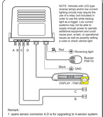
2. 2-sensor system, don't pull out plug A,D.
