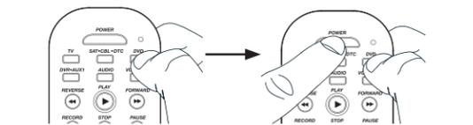
3. Wait until the remote's indicator LED comes on and stays on. Then release both keys.
