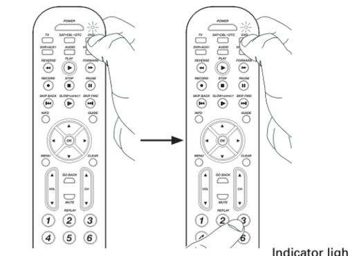
4. When you've finished entering the four-digit code, keep holding down the device key and look at the indicator light.
