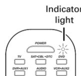
1. Press and hold the device key (TV, SAT•CBL•DTC, DVD, AUDIO, VCR•AUX2, DVR•AUX1) whose code you wish to retrieve. The indicator light turns on. Keep pressing the device key.
