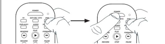
4. Wait until the remote's indicator comes on and stays on. Then release both keys.
