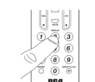
6. Point the remote directly at the front panel of the device you want to control. Press POWER on the remote and wait 2 seconds. The remote is testing a single code for your device's brand.
