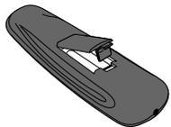
1. Remove the battery compartment cover.
