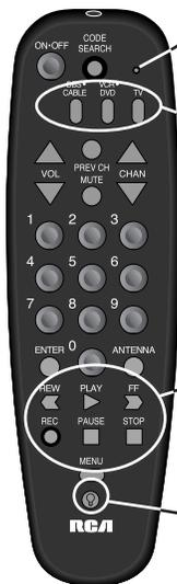
**Indicator Light**—flashes when a valid key is pressed to indicate the remote is working. Status of this light is important when you are programming the remote.
