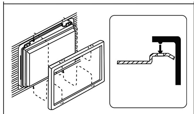
**NOTE: For proper operation of the CD/DVD player, the chassis must be mounted within 30° of horizontal. Make sure the unit is mounted within this limitation.**
