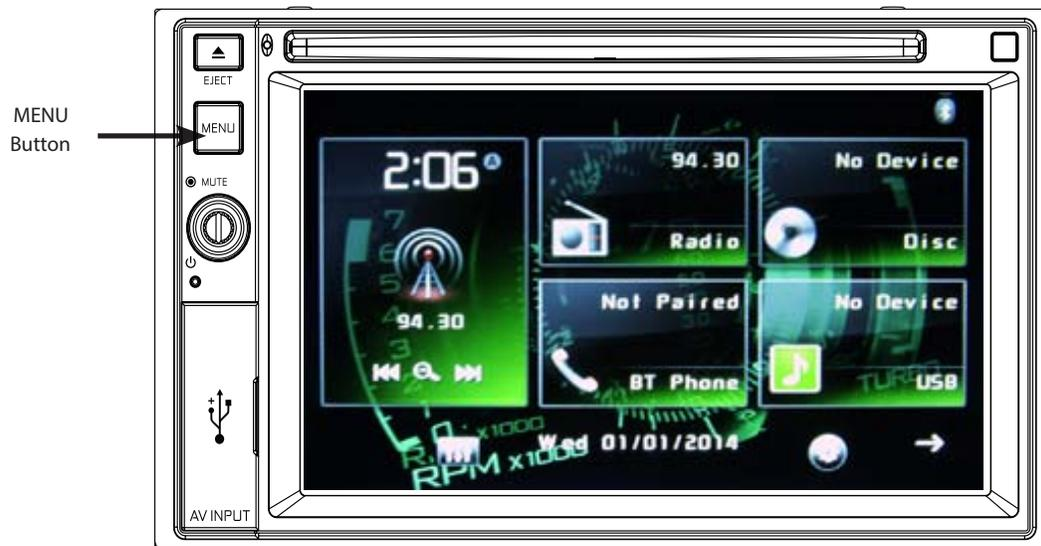
2. Touch the desired source icon on one of the two main menu screens. Screen 1 of 2: Radio, Disc, BT, USB. Touch page arrow (-->) at the bottom of the screen to access Screen 2 of 2: BT (Audio), Steering Wheel Control (SWC), AV-IN1, AV-IN2, or Camera.
