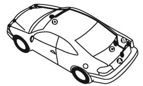
When mounting the camera make sure the surface in clean and oil free. Use the supplied angle wedges to adjust the sensor angle if needed. If the unit falses (beeps with no obstruction) adjust the angle upward away from the ground.
