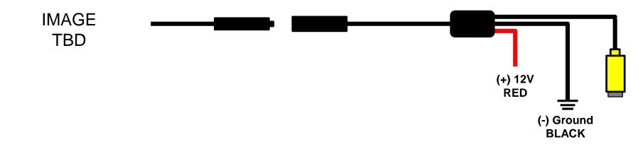
RED WIRE: Connect to 12V+ power source (ACC or IGN or REVERSE) BLACK WIRE: Connect to stable ground YELLOW RCA: Connect to input of designated video screen/interface
