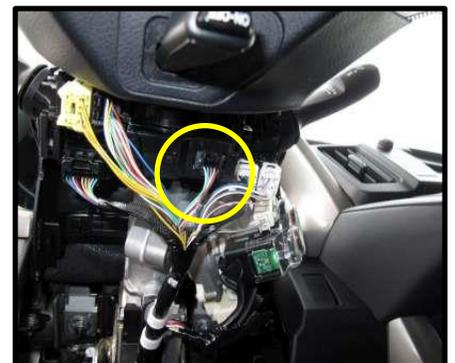
4. Mount or wire tie CAN BUS Module to side wall of the IP opening. Cables from button and CAN T Connectors should be routed around opening and secured. Route CAN BUS main cable to Main harness in lower kick panel. Make Main harness connections in lower kick panel. (Figure F4a-c)
