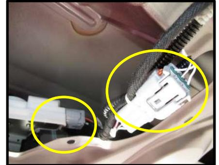
3. Mount buzzer (1901454235500) and switch harness (3140122001016) to rear tailgate in location that will not interfere with tailgate trim panel. This cable also routes into rear switch (PBB280020000). Install switch and cable. Continue routing cable to control box. (Figure E3a-b)
