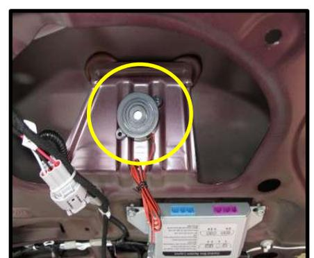
4. Route the main harness through the rubber gasket. Allow enough harness to extend towards rear of vehicle to reach Control box. **NOTE: use a wire puller to pull harness through gasket. Protect harness connectors by taping over them so they pass through easier.** (Figure E4)
