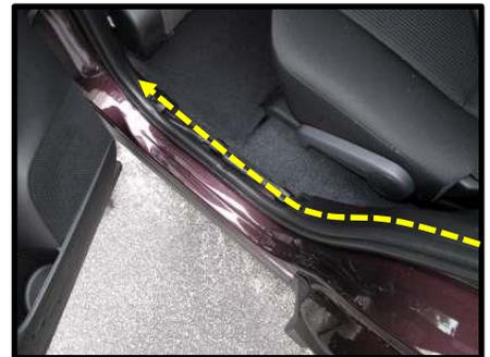
9. Continue routing cable forward tucked under lower B-pillar panel and into driver side sill area. (Figure E9a-b)
