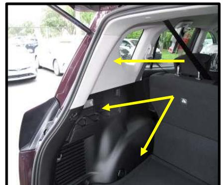
7. Remove headliner fasteners using a NRT to allow for harness routing. (Figure B7)
