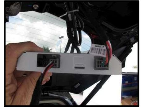
2. Use wire ties to clean up all routing making sure cables do not rattle or interfere with any other vehicle parts or operation.
