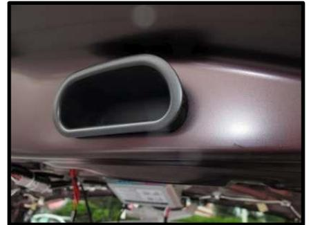
5. Pry rubber harness gasket away from liftgate and vehicle panel. (Figure B5)
