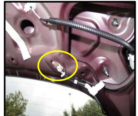
7. Now route main harness into vehicle. Continue routing main cable through gasket between headliner and over to rear side panel. Continue behind side interior panel or lower panel depending on routing preference. **DO NOT route harness where it may interfere with seat belt or air bags.** (Figure E7a-b)
