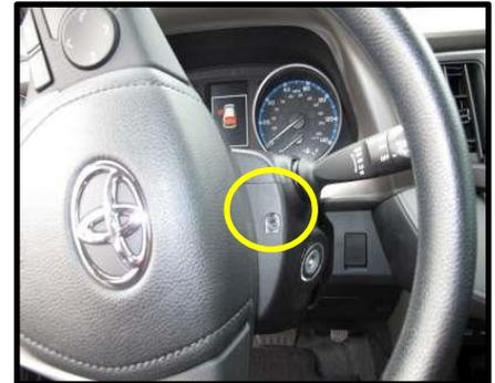
12. Using an NRT, separate the upper and lower half steering wheel trim panels. Remove lower panel. (Figure B12a-b)
