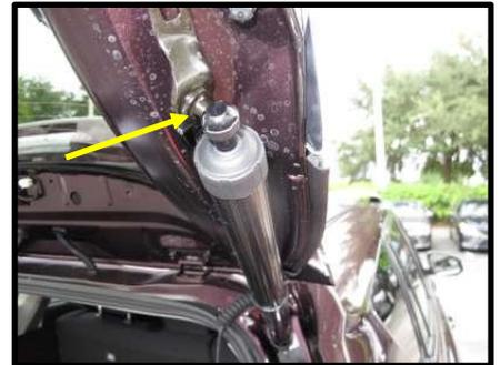
3. Pop out the factory bushing. Using a Razor knife, cut out the bushing from the rubber flap. (Figure C3a-b)
