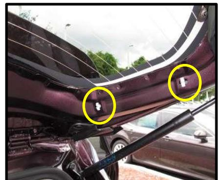
3. Using a NRT and hand, remove the large liftgate trim piece. (Figure B3)
