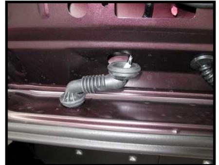
6. Remove rear driver side panels, upper or lower depending on preference of harness routing. (Figure B6)
