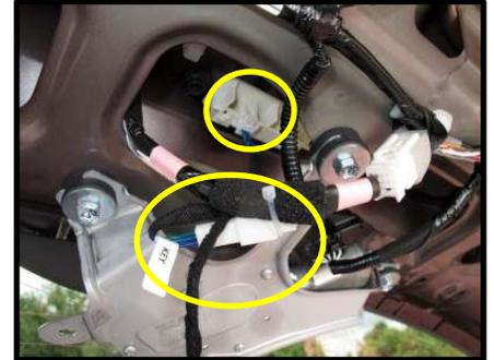
2. Locate Tailgate latch connector. Disconnect the connector and insert Lock T harness of 3110122001056. Connect the factory connector into the T-harness. Continue routing cable towards Control Box. (Figure E2a-b)
