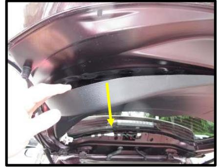
4. By hand, reach behind the handle insert on the Liftgate. Press on the upper and lower sides to push out the handle. (Figure B4a-b)
