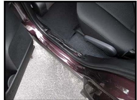
9. By hand, twist off plastic nut at front of kick panel trim. Pull up and remove 2-piece lower panel. (Figure B9a-b)
