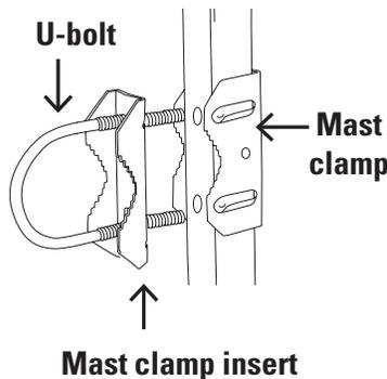
Find the U-bolt and mast clamp insert (see the illustration to the left). Put the U-bolt into the mast clamp insert with the teeth of the mast clamp insert facing the closed end of the U-bolt.
