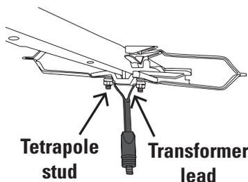
Use them to attach the transformer to the bottom of the antenna at the studs on tetrapole.
