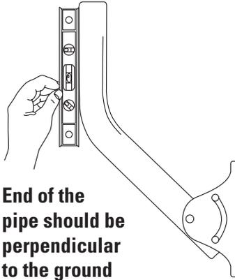
End of the pipe should be perpendicular to the ground (plumb)
