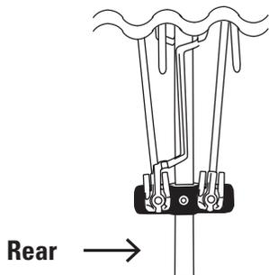
Starting from the rear of the antenna, unfold the elements on both the top and bottom of the antenna until they lock into place (as illustrated below). Make sure the elements are flat and parallel to each other when you've finished.
