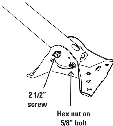
Find the end of the mounting pipe with holes on the sides for screws. Insert this end into the middle of the foot as illustrated here. Then insert the 2-1/2" screw through the foot and pipe as shown. Screw the 1/4" hex nut onto the end of the screw to hold the pipe and foot together. *Don't tighten the nut completely yet.*
