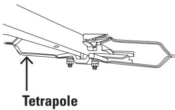
Make sure the tetrapole locks into place. Do not attach the downlead yet!
