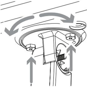
You can also adjust the antenna's orientation on the antenna itself. On the antenna's underside, next to the arm, there are two screws. Loosen these just enough so that you can rotate the antenna on the arm. Once you've found the orientation you want, tighten these screws.
