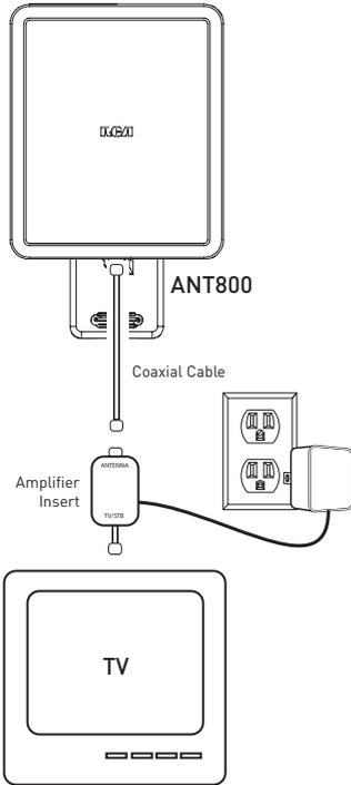
1. Run an RG6 coaxial cable from the antenna towards your television set. Connect the RG6 coaxial cable to the ANT jack on the supplied amplifier insert.
