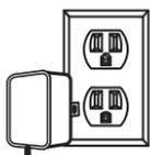
Plug the power cord for the antenna's power injector into a standard AC outlet. Don't connect it to your TV yet.
