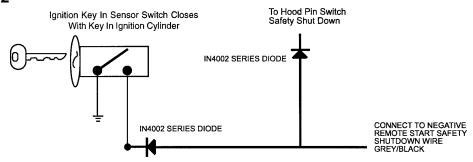
To connect to the key in sensor circuit as shown for method 2:
