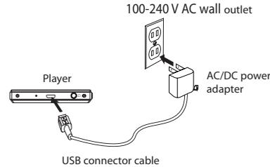
\* Use only USB power adapter conforming with USB Battery Charging Specifications 1.2 or above (not supplied)
