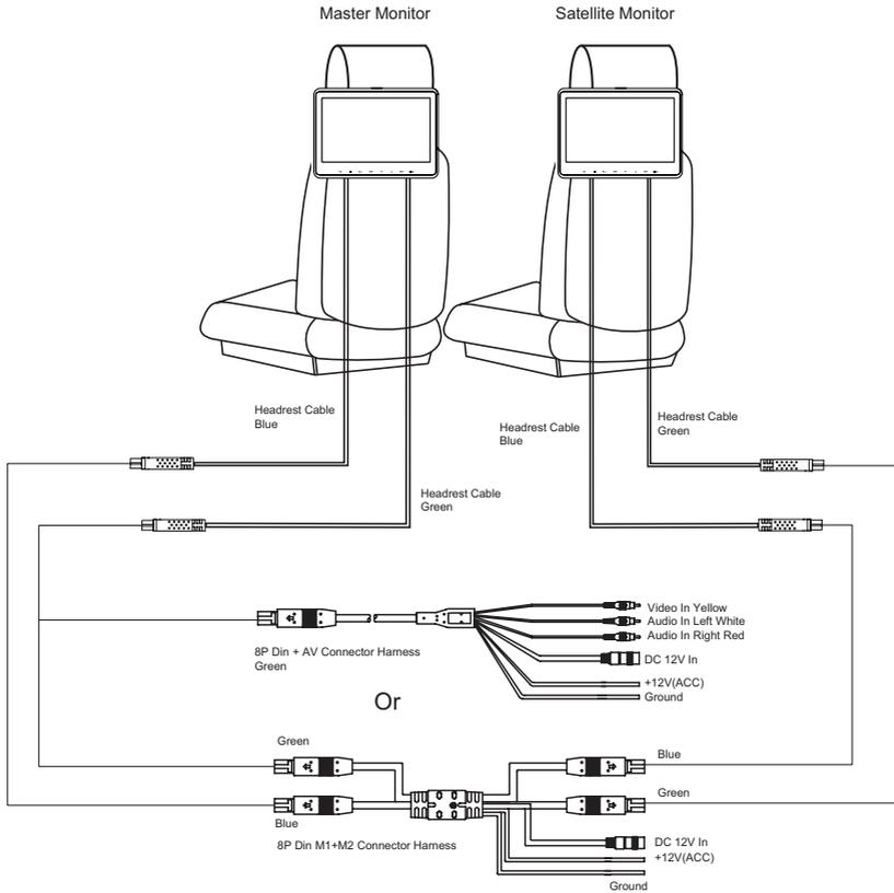
**NOTE: Please do not use incorrect cable harness on the monitor system because user will lose some functions if installed incorrectly.**
