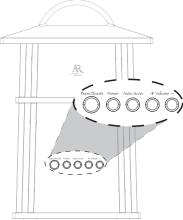
1. Press the Power button on the back of the speaker to turn it on.
