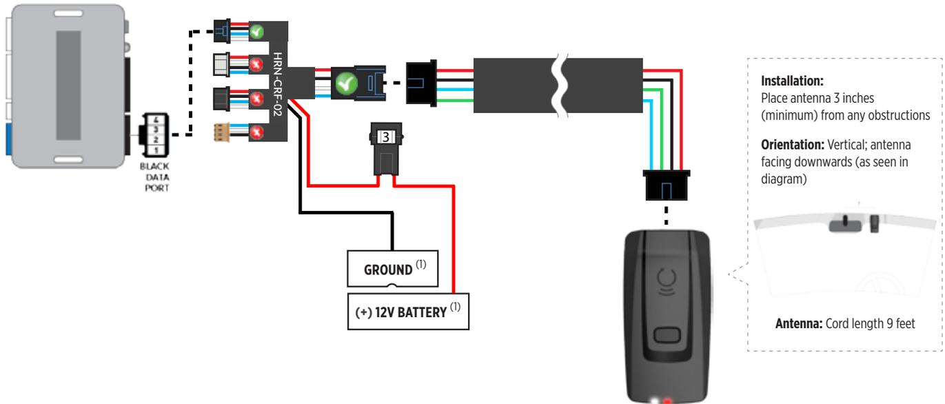
(1) Connect when using with FL-CAN.
