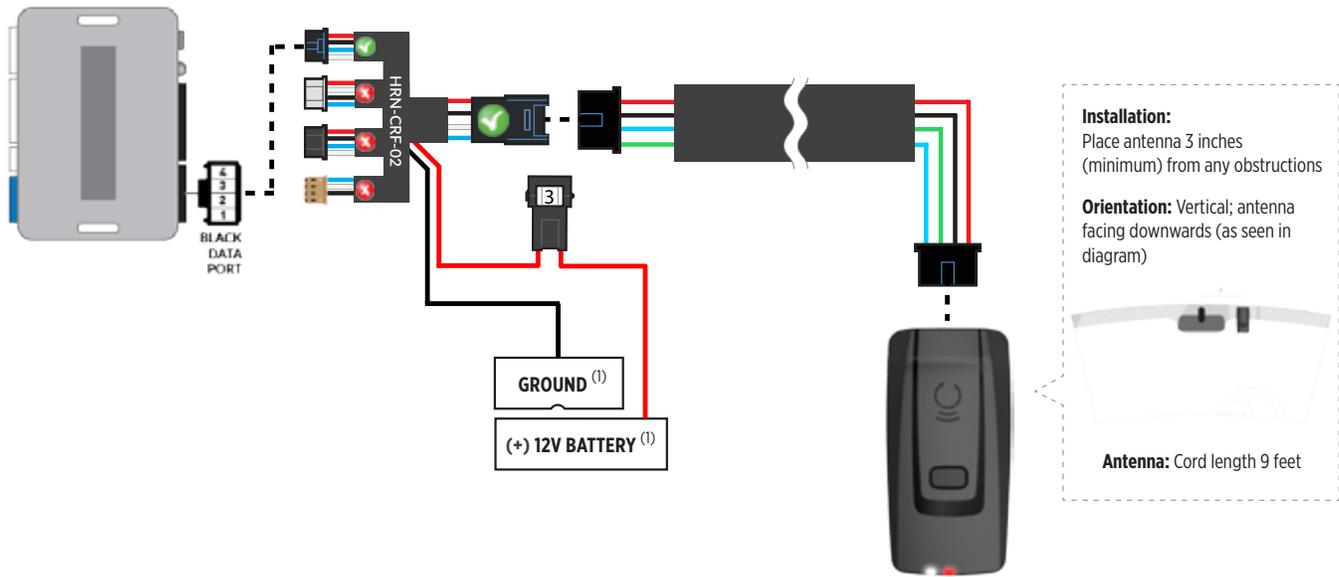
(1) Connect when using with ADS-AL-CA.
