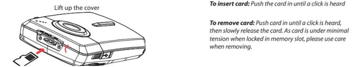
As the memory card is small in size, it is recommended to use a **small coin** to help insert or remove it.
