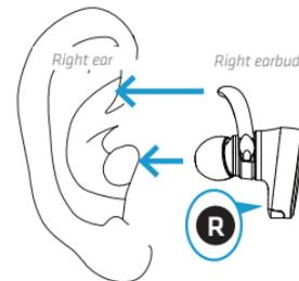
Unplug the USB charging cables when the earbuds are charged. Place each earbud in its assigned ear (marked R or L on the inside of each bud).
