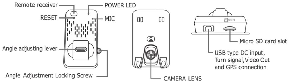
To clean the camera lens, use a soft, dry clean cloth, or specially made camera lens wipes **ONLY**. Periodic cleaning is required to maintain proper operation. Do **NOT** move the lens angle when cleaning.
