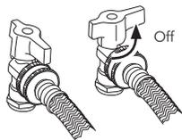
Turn each valve 90-degrees counter-clockwise to turn it off. Place a bucket and towels under the shut-off valves before you remove the hoses.
