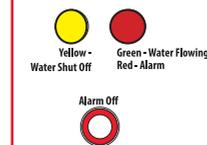
If the sensor senses water, the alarm sounds and the valves close. The yellow and red indicators on the control box start flashing. You will also receive a notification on your phone saying "Device has been triggered. Automatic shut-off activated."
