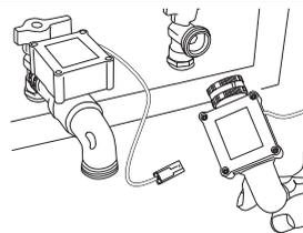
Remove the plastic protectors from both ends of each automatic shut-off valve. Make sure the rubber o-rings are seated properly (flat) inside each hose fitting.
