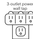
If both power outlets are in use (by the washer and dryer, for example), use the included 3-outlet power wall tap to provide additional outlets.
