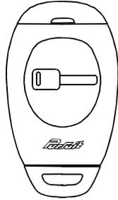
1. To start the vehicle, press and release the transmitter button two times within 2 seconds. The vehicle will start and remain running for the pre-programmed 5,10,15,20 minute run cycle. As a visual indication, the parking lights will flash or remain on depending on the setting by your installation center.
