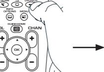
4. When you've finished entering the five-digit code, keep holding down the device key and look at the POWER key.
