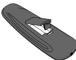
1. Remove the battery compartment cover.
