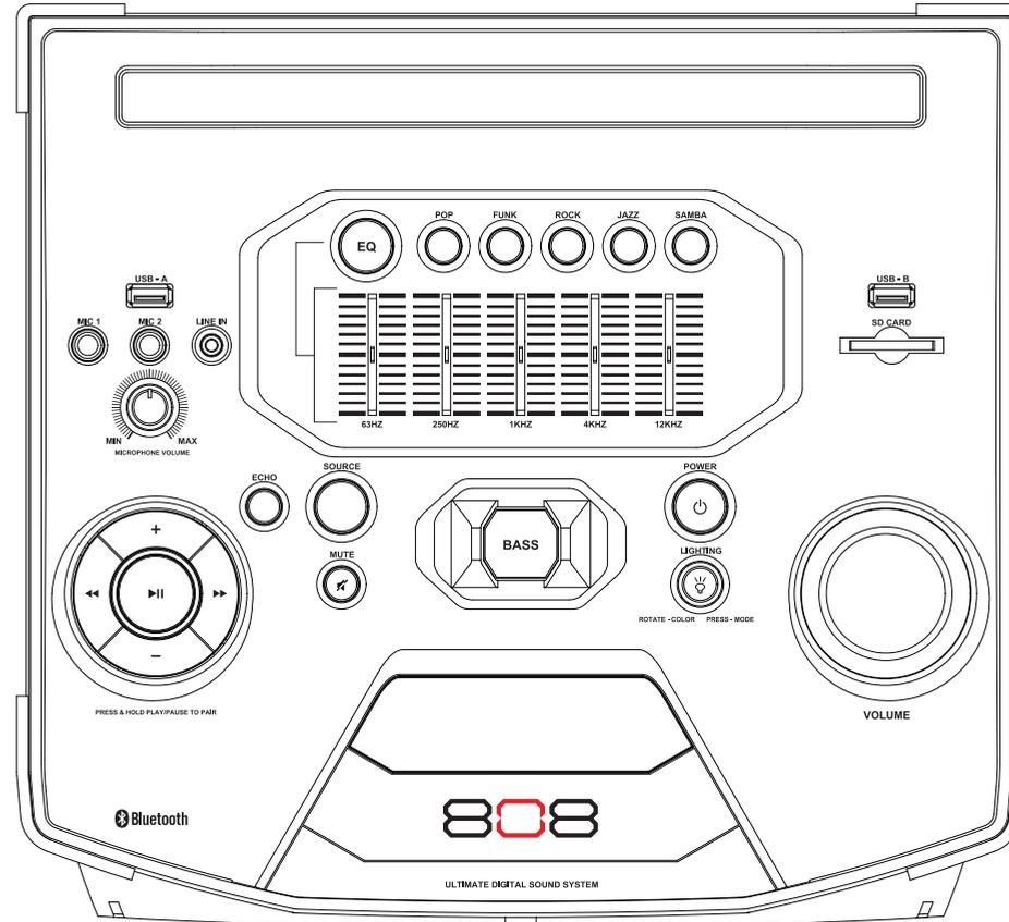
**▶|| button** starts or pauses playback in USB, SD, or Bluetooth modes. In radio mode, scans for stations and stores presets (press and hold). In Bluetooth mode, press and hold to start pairing to a new Bluetooth device.
