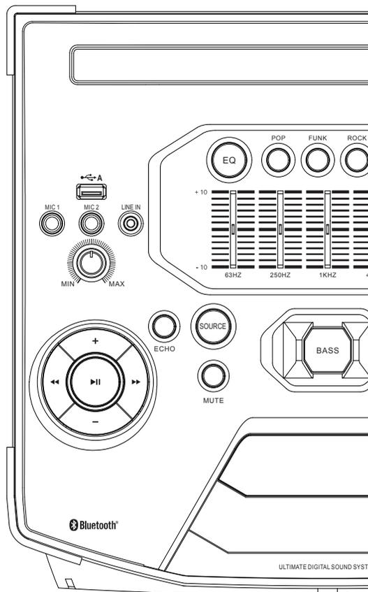
**▶|| button** starts or pauses playback in USB, SD, or Bluetooth modes. In radio mode, scans for stations and stores presets (press and hold). In Bluetooth mode, press and hold to start pairing to a new Bluetooth device.
