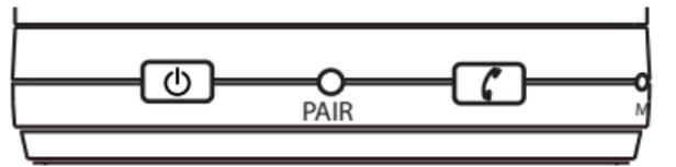
**CALL** button has two functions: (1) it turns the speaker on and off (press and hold) and (2) puts the speaker into pairing mode (short double-press) to connect to a new Bluetooth device.
