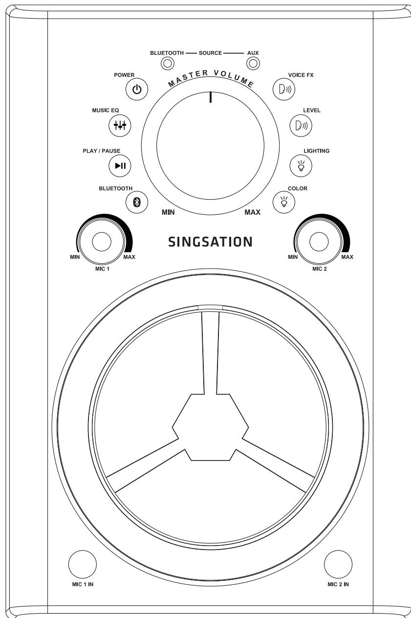
**BLUETOOTH indicator** shows the Bluetooth status of the Singsation Classic (solid is connected; fast flashing means pairing, and slow flashing means not connected).
