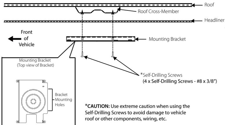
**WARNING:** Any use of a mounting substrate other than the supplied bracket may result in performance issues. The supplied bracket was designed to ensure this Mobile Video System is properly installed without adding any strain or stress to the system which could result in unit operation problems.
