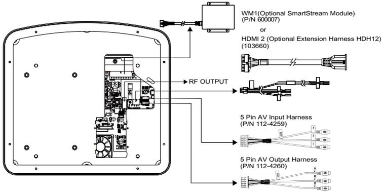
**NOTE: The Hidden 24 Pin connector only allows connection of either optional SmartStream Module (WM1) or HD/USB Extension harness (HDH12).**
