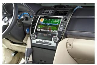
The 2012 Camry System includes features like Pandora internet radio control (when available), built-in Navigation package with state-of-the-art iGo Primo software featuring lane assist, Navteq US and Canada maps plus 11 million POIs and 3D landmarks and building graphics. The system also offers 19 on-screen display languages, and text-to-speech recorded voice guidance in English, French and Spanish.
