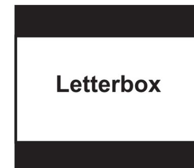
This system uses a widescreen 16:9, or 1.85:1 display - the same aspect ratio as high-definition televisions. This means that when viewing widescreen DVD's, these black bars are either non-existent, or greatly minimized.
