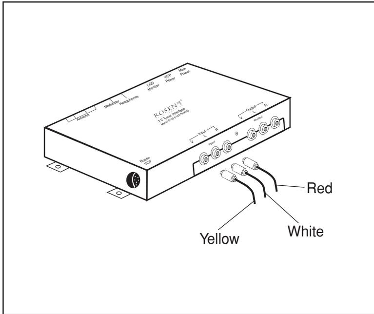
Connecting game systems or camcorders is as easy as matching the colors of the RCA plugs on the device to the colors on the INPUT jacks on the TV Tuner Interface.
