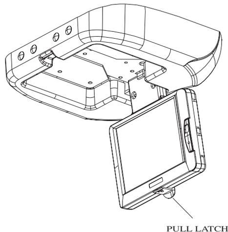
The push button on the overhead console releases the Auto Video™ screen just far enough so that it can easily be positioned for optimal viewing. This action sends power automatically to all the system components. The screen will display the last video signal chosen. (see 2-6 configuring your system)
