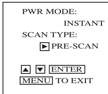
Choosing the **OPTIONS** menu (diagram 1, above) and moving into the **CONFIGURE** menu will allow you to set the **SCAN TYPE** to either **RT SCAN** (Real Time Scan), or **PRE-SCAN**.
