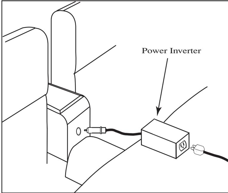
Some video game systems, camcorders, and other video devices require 120 VAC "household" current instead of the 12 VDC supplied by your vehicle. These devices require the use of an AC power inverter (not a *converter*) to change the vehicle's 12 VDC to 120 VAC.
