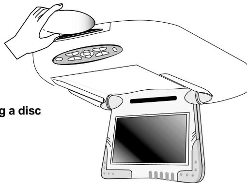
Inserting a disc
