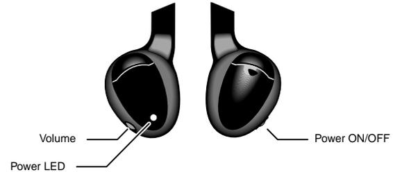
To turn the headphones on and off, push the Power ON/OFF button on the right ear piece. The Power LED on the left ear piece indicates when headphone power is on. Power turns off automatically after three minutes of no audio to preserve battery life. To adjust the headphone volume, rotate the thumb wheel switch on the headphones.
