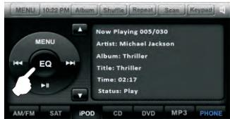
Touch the EQ button when the play information is displayed and it will launch the spectrum display if the spectrum is enabled.
