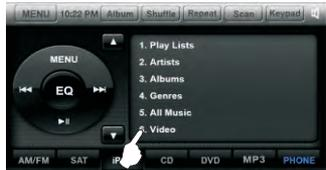
While in video play mode, touch the screen to open the iPod control panel.
