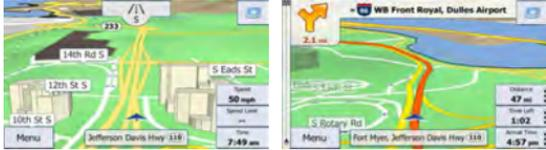
Tap any of the data fields to suppress others and display only the selected one. The data fields are different when you are navigating an active route and when you have no specified destination (the orange line is not displayed).
