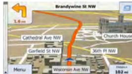
There is a field in the top left corner that displays the next maneuver. Both the type of the event (turn, traffic circle, exiting freeway, etc.) and its distance from the current position are displayed.
